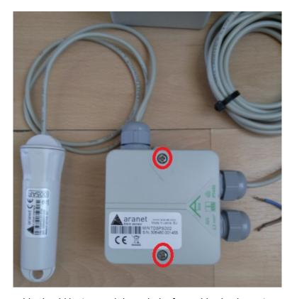
2) Then power cable should be inserted through the free cable gland opening:
