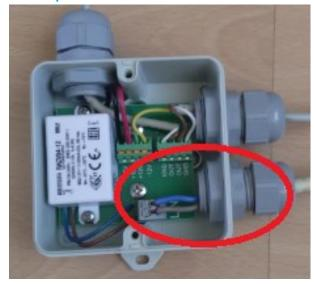
Once the AC power connection is made, the junction box can be closed, gland for the power cable tightened and AC power turned on for the sensor.
