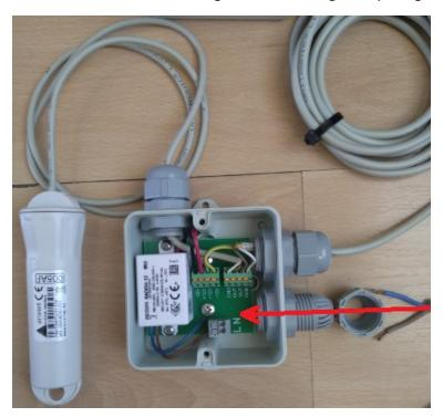
3) And finally connecting power cable line (phase, "hot") wire to L clamp on the sensor board and neutral ("cold") wire to N clamp:
